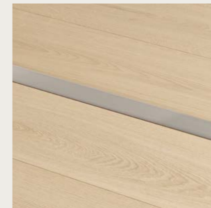
EXPANSION PROFILE 2000 × 31 × 10 mm To cover the expansion gap between two floors of the same height. Surface: aluminium. SFEXPSILV | SFEXPCOFF | SFEXPCLAY | SFEXPCHAM | SFEXPBLACK
